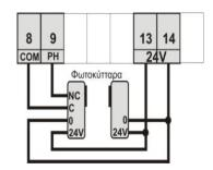
**Photocell operation:** When the door closes and the photocell beam is cut-off, the door stops immediately and automatically activates the open function. If the photocell beam is cut-off, the door never closes.
