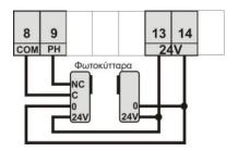
**Photocell operation:** When the gate closes and the photocell beam is cut-off, the gate stops immediately and automatically activates the open function. If the photocell beam is cut-off, the gate never closes.
