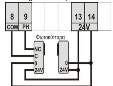
**Photocell operation:** When the door closes and the photocell beam is cut-off, the door stops immediately and automatically activates the open function. If the photocell beam is cut-off, the door never closes.
